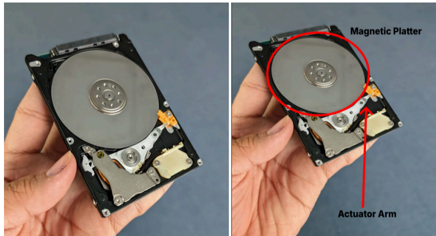
Figure 3.3: The inside of an HDD, with annotations explaining the parts.
