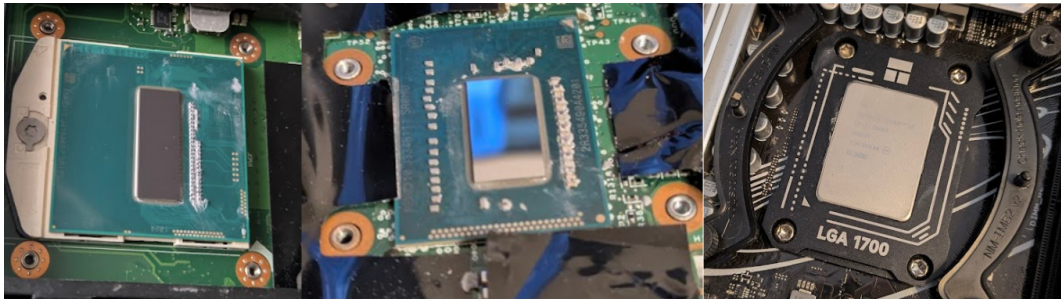
Figure 3.11: An Laptop CPU in a socket, an Intel Core i7-4712MQ, a Laptop CPU directly soldered on the motherboard, an Intel Core i7-3520M, and a desktop Intel Core i7-14700KF.
