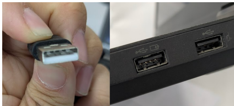
Figure 2.2: The connector and port of USB-A
