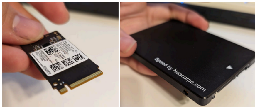
Figure 3.5: Two SSDs, one using the NVMe interface and one using SATA. Both are internal drives meant to be mounted into a computer's casing.
