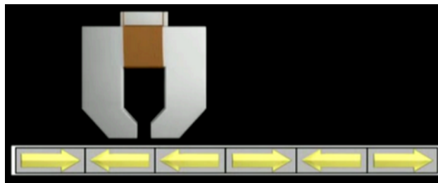
Figure 3.4: What the magnets inside an HDD looks like.
