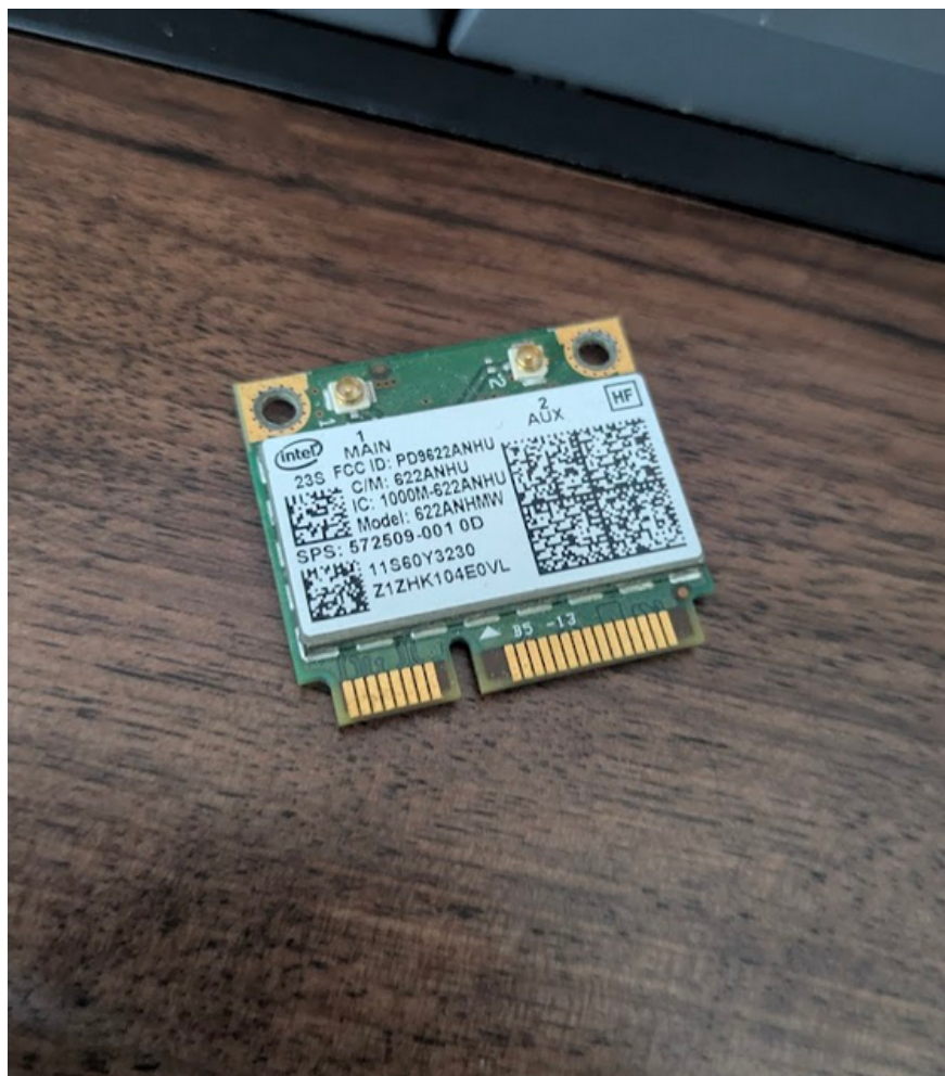
Figure 3.15: A network interface card used in a laptop.
